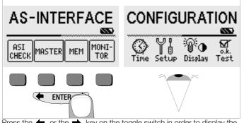
Press the  $\blacklozenge$  or the  $\clubsuit$  key on the toggle switch in order to display the desired measuring function, device settings or database functions.
