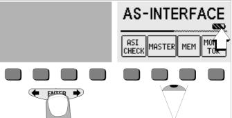
The instrument can be switched on by pressing any key.
