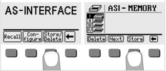
After activating the Store/Delete key once, the desired memory address (I, II, III or IV) must first be selected with the Next key, to which the slave addresses which are now in RAM are to be stored. After activating the Store key a second time, a list of all stored slave addresses is generated. If the Store key is activated again, a menu appears for the entry of a new system name, or a new AS-i bus name for the previously selected memory address.
