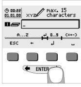
Display the desired alphanumeric character by pressing the ← or the → key at the toggle switch and select it with the corresponding softkey. Control characters are entered in the same way and have the following meanings:
