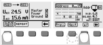
After initializing the SLAVE CHECK function, slave addresses 0 through 15 are displayed along with the abbreviated data from the slave with the lowest address. The display can be switched back and forth between address ranges 0 through 15 and 16 through 31 with the  $\leftarrow$  or the  $\rightarrow$  key at the toggle switch. The desired slave address from either of the address ranges is selected with the Prev. or Next key, and is acknowledged with the  $\downarrow$  key.
