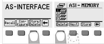
After activating the Store/Delete key, a previously stored bus configuration or the corresponding memory address can be selected with the Next key.
