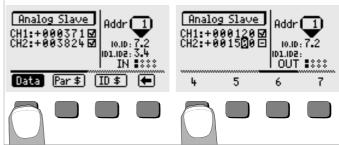
Analog data channels can be activated for output modules with the Data key, and transmitted to the slave after acknowledgement. Numerals which do not appear initially can be displayed by pressing the  $\leftarrow$  or the  $\rightarrow$  key at the toggle switch. Each time a numeral is selected, the cursor moves one place to the right.
