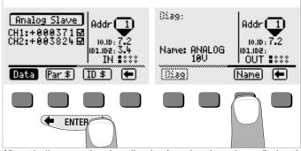
After selecting an analog slave, the slave's analog channels are displayed at the left, and abbreviated slave data appear at the right. The display can be switched to the diagnosis string (if available), as well as to the name entry menu and back to the main menu with the  $\blacklozenge$  and  $\clubsuit$  keys at the toggle switch. After activating the Name key, the instrument is switched to the alphanumeric entry mode as described in chapter 7.3.
