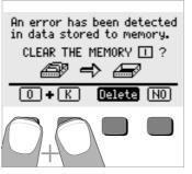
These data can be saved to a PC via a PC interface and reconfigured if desired. Reconfigured data can be uploaded from the PC to the METRAtest 36ASi as well. If an error is detected in the memory, the user is asked whether the defective memory should be cleared and thus re-initialized. For example, errors may occur after the rechargeable battery has been replaced. Refer to chapter 7.4 regarding memory clearing.
