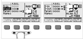
The hourglass and the arrow indicate transmission to the slave and updating of the **D-in** inputs. Key operations are disabled during transmission of parameters and data. This is indicated by means of dashed softkeys.
