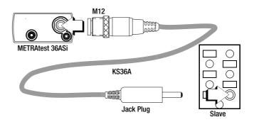
The necessary connections have now been established, and addressing can begin with the METRAtest 36ASi addressing and test instrument.
