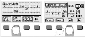
After initializing the Set Slave function, slave addresses 0 through 15 are displayed along with the abbreviated data from the slave with the lowest address. The display can be switched back and forth between address ranges 0 through 15 and 16 through 31 with the ← or the → key at the toggle switch. The desired slave address from either of the address ranges is selected with the Prev. or Next key and is acknowledged with the ↓ key. The slave profile appears at the display.
