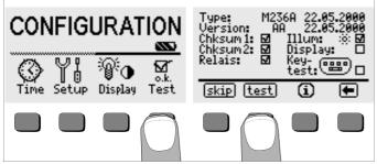
The self-test is started from the main menu with the Test key. The test has a duration of several minutes. The following information is displayed in the two headers:Type:Device type / date of last calibrationVersion:Software version and issue date
