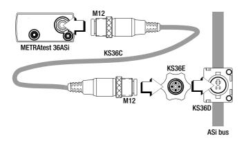
The necessary connections have now been established, and testing can begin with the METRAtest 36ASi addressing and test instrument.
