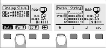
Beyond this, the parameter string (Par \$) can be queried or edited, and the ID string (ID \$) can be read out. After the parameter string has been edited, the new values are transmitted directly to the slave. Switching is possible between bytes 00 through 02, 03 through 05, 06 through 08 and 09 through 11 with the Prev. or Next key, or with the  $\bigstar$  or  $\clubsuit$  key at the toggle switch.
