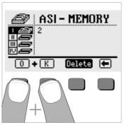
A security query is displayed if the Delete key is activated from the ASI-MEMORY menu: The 0 and K keys must be activated simultaneously in order to acknowledge deletion of the contents of the memory, or the selected memory address.
