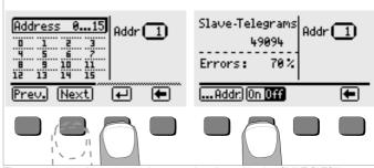
The error quota for a single slave can be viewed in the SLAVE CHECK sub-menu by selecting the desired slave address.
