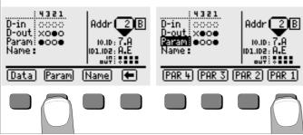
If valid data and parameters have been entered completely, they are transmitted to the slave by activating the **ENTER** key. Input data are updated cyclically by the slave.
