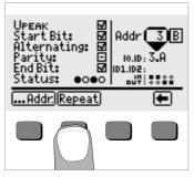
If only one slave has been connected to the bus, the above described selection menu does not appear. The slave's telegram data are displayed, which allows for conclusions regarding possible data transmission errors. Measurement can be repeated with the Repeat key.
